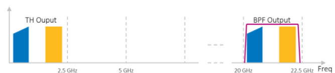
Figure 3 - Receive path TH ( f_s = 5 GHz) sub-sampling of 2.5 GHz bandwidth signal (on a 21.25 GHz carrier).
