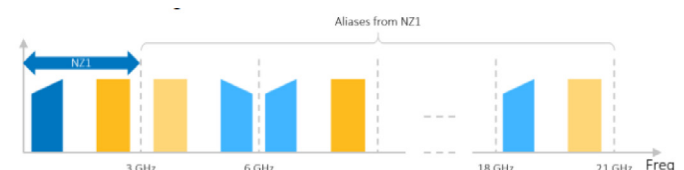
Figure 4 - Synthetic RF signal generated in NZ1 and aliased into higher order Nyquist zones ( f_s = 6 GHz).
