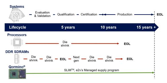
Figure 3 - System and product lifecycles vary considerably adding to the challenge of selecting key components in long life projects
