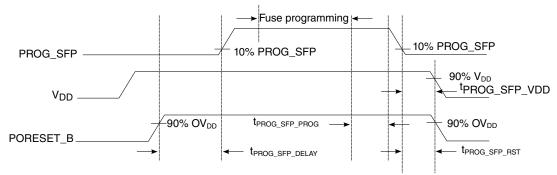
Note: PROG\_SFP must be stable at 1.8 V prior to initiating fuse programming.
