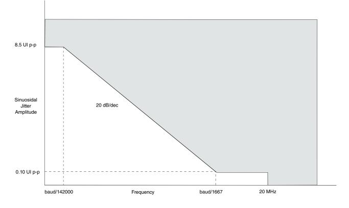
This table defines the receiver AC specifications for serial RapidIO operating at 5 GBaud. The AC timing specifications do not include RefClk jitter.
