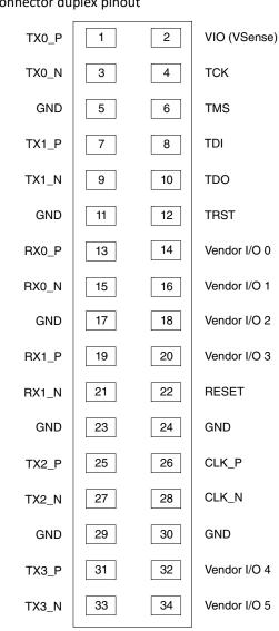
Figure 4-12. Aurora 34 pin connector duplex pinout
