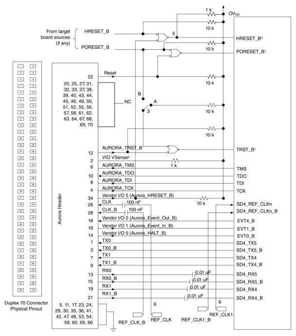
Figure 4-13. Aurora 70 pin connector duplex interface connection
