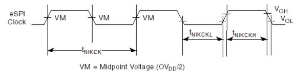
This figure represents the AC timing from Table 3-28 in master mode (internal clock). Note that although the specifications generally reference the rising edge of the clock, these AC timing diagrams also apply when the falling edge is the active edge. Also, note that the clock edge is selectable on eSPI.
