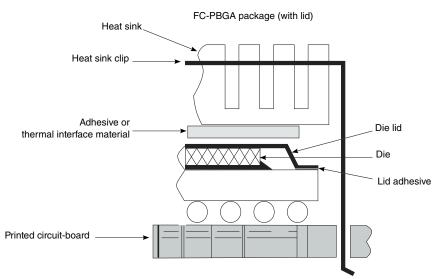
The system board designer can choose between several types of heat sinks to place on the device. There are several commercially-available thermal interfaces to choose from in the industry. Ultimately, the final selection of an appropriate heat sink depends on many factors, such as thermal performance at a given air velocity, spatial volume, mass, attachment method, assembly, and cost.
