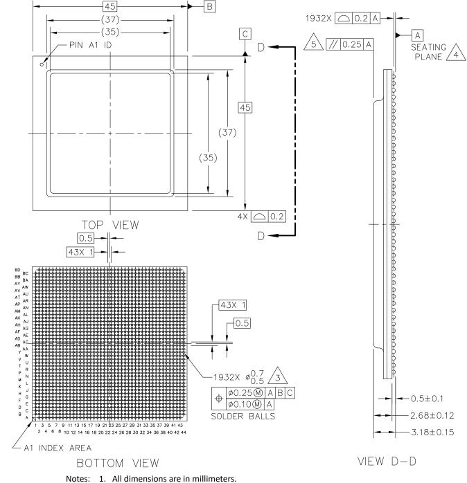
Figure 6-1. Mechanical dimensions of the ROHS FC-PBGA with full lid
