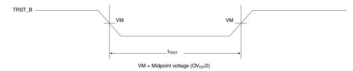
This figure provides the boundary-scan timing diagram.
