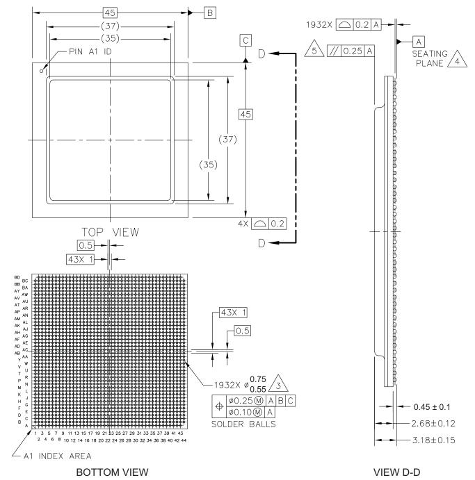
Figure 6-2. Mechanical dimensions of the SnPb FC-PBGA with full lid
