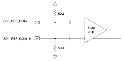
The characteristics of the clock signals are as follows:
