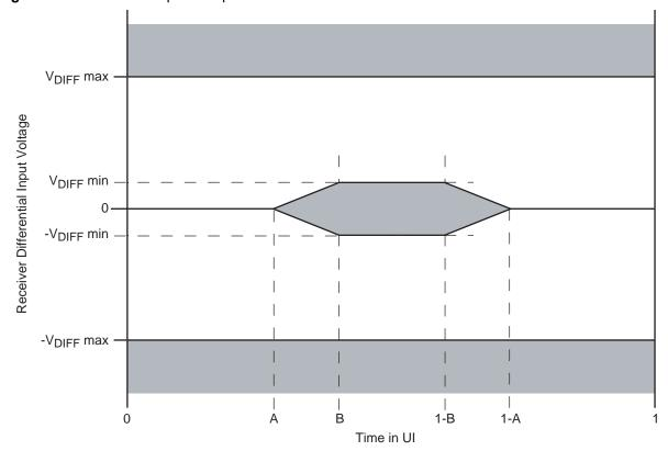
Figure 18-4. Receiver Input Compliance Mask
