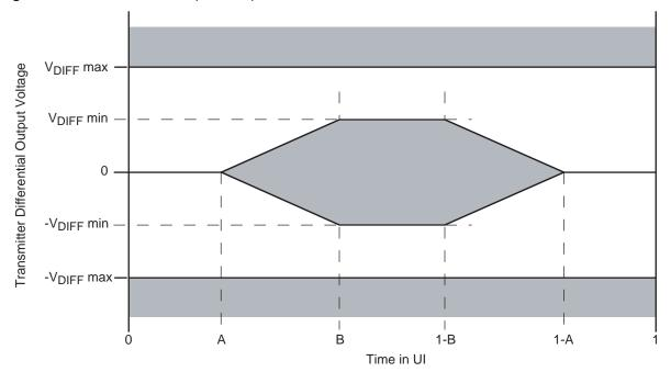
Figure 18-2. Transmitter Output Compliance Mask
