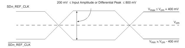
Figure 16-5. Single-Ended Reference Clock Input DC Requirements
