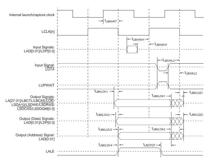
Note: In PLL bypass mode, LCLK[n] is the inverted version of the internal clock with the delay of t<sub>LBKHKT</sub>. In this mode, signals are launched at the rising edge of the internal clock and are captured at falling edge of the internal clock withe the exception of LGTA/LUPWAIT (which is captured on on the rising edge of the internal clock).
