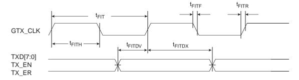
Figure 8-2. FIFO Receive AC Timing Diagram
