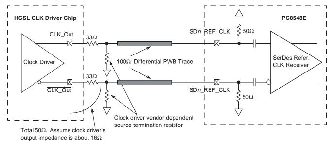
Figure 16-7 shows the SerDes reference clock connection reference circuits for LVDS type clock driver. Since LVDS clock driver's common mode voltage is higher than the PC8548E SerDes reference clock input's allowed range (100 to 400mV), AC-coupled connection scheme must be used. It assumes the LVDS output driver features  $50\Omega$  termination resistor. It also assumes that the LVDS transmitter establishes its own common mode level without relying on the receiver or other external component.
