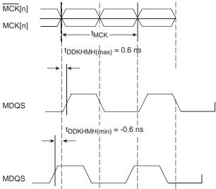
Figure 6-2 shows the DDR SDRAM output timing diagram.
