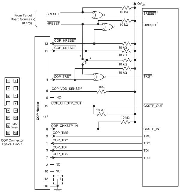
Notes: 1. The COP port and target board should be able to independently assert HRESET and TRST to the processor in order to fully control the processor as shown here.
