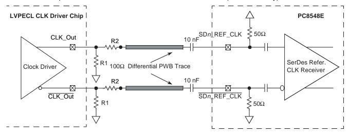
Figure 16-9 shows the SerDes reference clock connection reference circuits for a single-ended clock driver. It assumes the DC levels of the clock driver are compatible with the PC8548E SerDes reference clock input's DC requirement.
