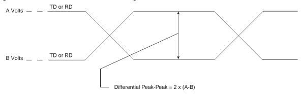
To illustrate these definitions using real values, consider the case of a CML (Current Mode Logic) transmitter that has a common mode voltage of 2.25V and each of its outputs, TD and TD, has a swing that goes between 2.5V and 2.0V. Using these values, the peak-to-peak voltage swing of the signals TD and TD is 500 mV p-p. The differential output signal ranges between 500 mV and –500 mV. The peak differential voltage is 500 mV. The peak-to-peak differential voltage is 1000 mV p-p.
