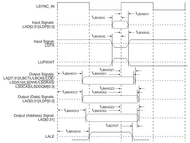
Table 10-5 describes the timing parameters of the local bus interface at BV<sub>DD</sub> = 3.3V with PLL disabled.
