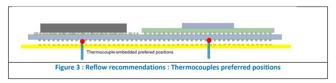
Note: Mechanical samples can be provided to tune the reflow process and the position of the thermocouples.
