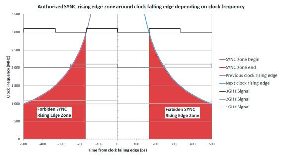
5. To correctly perform the synchronization procedure, the falling edge SYNC pulse should be synchronized with the falling edge of the clock.
